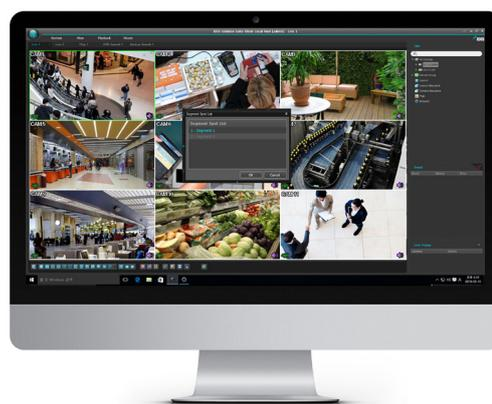
When a user changes the NVR system time to the past, video data for the overlapped time period is recorded in different segments. This enables video data for the overlapped time to be searched in a different time set and prevents any possible loss of video data or discrepancy on a time-based search.
