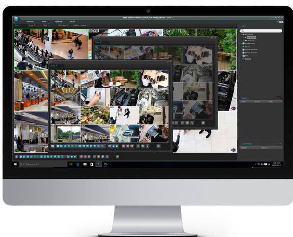
All control panels (Live, Playback, Event Search, Health, Report) operate based on a tab that is fully functional itself. Each tab can be detached and can be placed on the secondary monitor for a multi-monitor environment.
